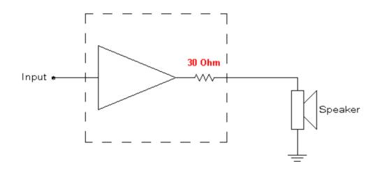
Here 30 Ohm for Current amp is the very minimum. Can you see there is a pattern? The type of amplifier is directly referenced to that of its output impedance. It changes, indeed *determines* the way the amplifier delivers power to the speakers.
