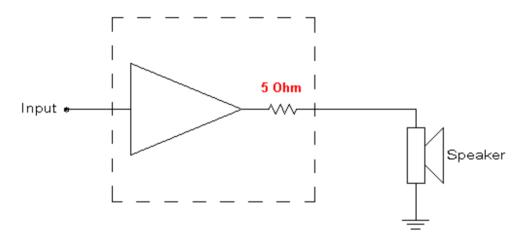
**3.** The Current Amp - the output impedance is many times that of the loudspeaker.
